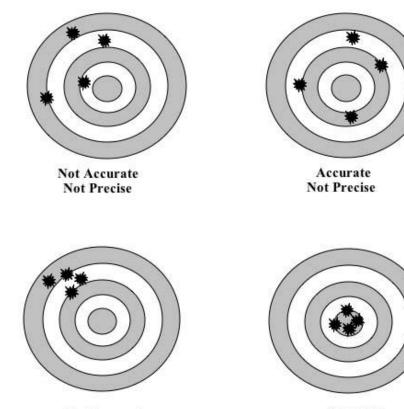
Not Accurate Precise Accurate Precise
