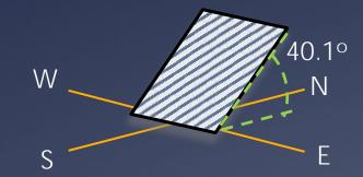
Example: Latitude of Boulder, Colorado is 40.1° so solar water heater is 40.1° from the ground facing South
