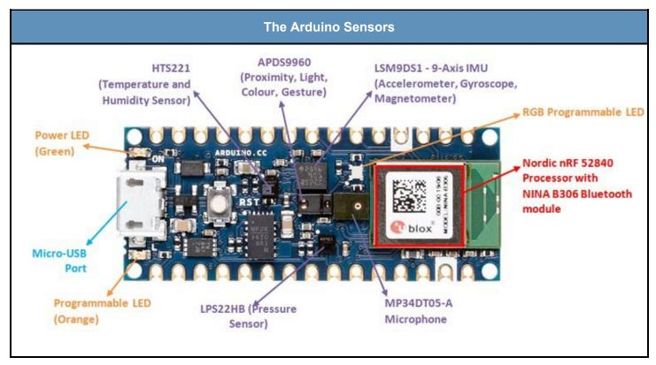
The student should circle the microphone as the ears, temperature & humidity sensor as fingers, and the proximity, light, color, and gesture sensor as eyes.
