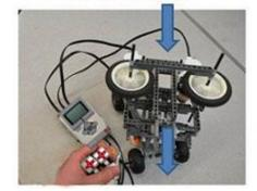
Display shows power value that changes with the press of a button
