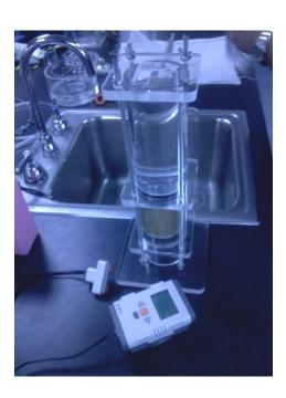
Permeameter with ultrasonic sensor and EV3 to measure water volume and time
