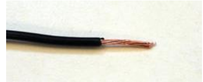
A stripped wire.
