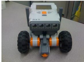
Connect: 2 gray axle-LEGO connectors to NXT brick using blue connectors; then connect touch sensor using black long connector as shown; set second touch sensor.
