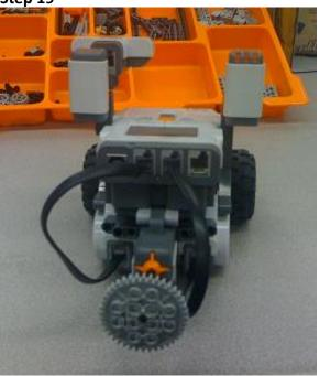
Obtain: port-sensor/motor wires and connect each motor/sensor to appropriate ports.
