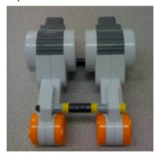
Obtain: 2 motors, 3 small black axles, 3 yellow thin washers, 1 black axle connector, 2 gray washers. Connect as shown above.
