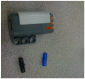
Connect the sound sensor and light sensor in the same manner. Obtain: 1 sound sensor, 1 blue connector and 1 black connector as well as 1 light sensor, 1 blue connector and 1 black connector.
