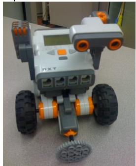
Obtain: touch sensor pieces from Step 13, 2 medium wheels, 1 large gear, and 3 black medium axles. Connect touch sensor as shown in Step 13; connect medium wheels with medium axle and gear with medium axle, as shown above.
