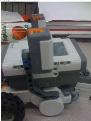
Connect sound sensor with blue and black connectors to angle, as shown. Do the same for the light sensor on the other side.
