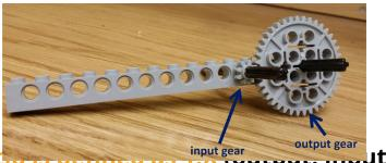
In this case, the gear ratio is defined as the number of teeth, Notice that this is in the same ratio as the number of teeth, that is, 8:40 or 1:5.
