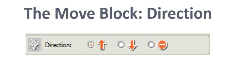
"Direction" controls which way the motors are set to rotate.
