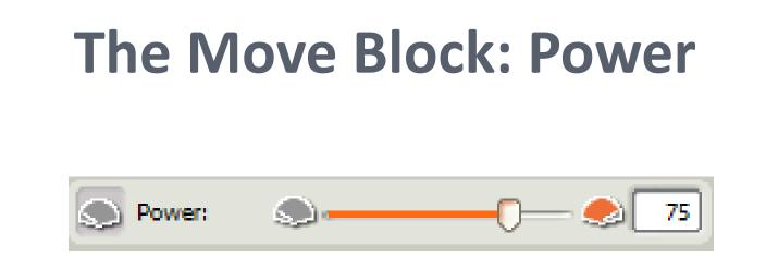
o The Power setting controls how fast the motors turn.
