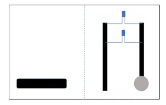
14. Put a red LED and a blue LED on the same battery. Which light is brighter? Why do you think one is brighter than another? The two LEDs are made from different materials. One takes more energy than the other to make the LED light. (This is called a band gap in semiconductor physics). Which one do you think takes more energy? If you were a stream of electrons coming from a battery do you think you would go to the light the LED that takes more energy or less?
