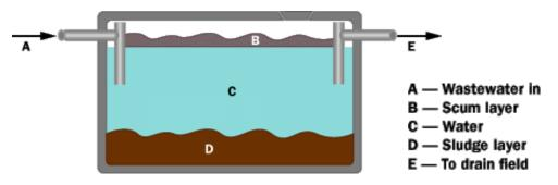
In this side-view drawing of a septic tank, you can see three layers. Anything that floats rises to the top and forms a layer known as the **scum layer**. Anything heavier than water sinks to form the **sludge layer**. In the middle is a fairly clear water layer that contains bacteria and chemicals (such as nitrogen and phosphorous that act as fertilizers), but is largely free of solids.
