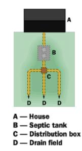
A septic system is usually powered by gravity alone. Water flows down from the house to the tank, and then down from the tank to the drain field. It is a completely **passive system**.
