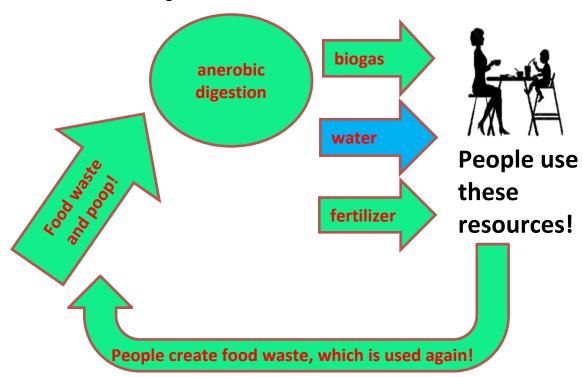
Anaerobic digestion's main product is gas. Biogas is usually ~70% methane (flammable!) and about 30% CO<sub>2</sub>. Natural gas, which may be piped into your house, is ~90% methane.
