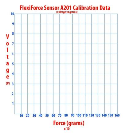
Instructions: Now that you know the best fit line, use it to calculate the minimum force required to crack an egg. The goal is to progressively add pressure to the egg, record the voltage and then calculate the pressure using the line of best fit.
