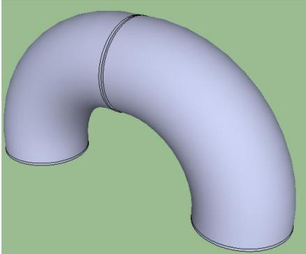
A 3D CAD model of a 180-degree return pipe bend, showing a smooth, U-shaped transition in a light blue pipe against a green background.                                                                    | <p><b>0.2</b></p>  |
