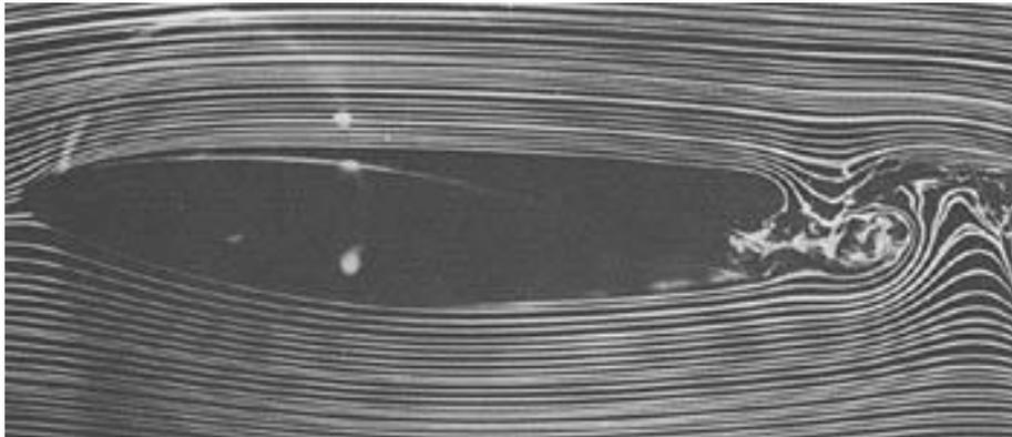
**Figure 1. Streamlines of smoke around an airplane wing in a wind tunnel.**
