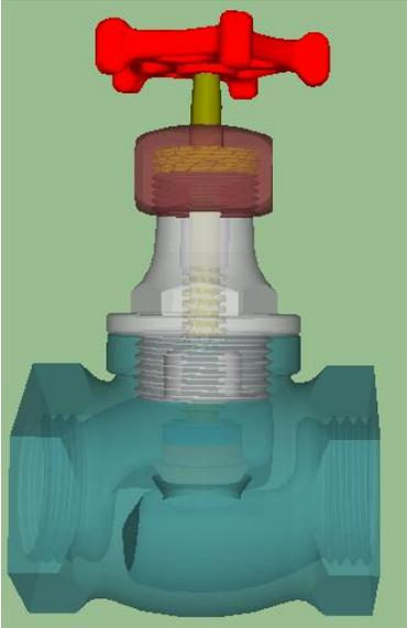
A 3D cutaway model of a globe valve in the fully open position. The valve body is teal, the stem is grey, and the handwheel is red. The internal flow path is visible, showing the valve is open.          | <p><b>10</b></p>   |
