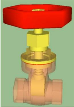
A 3D cutaway model of a gate valve in the fully open position. The valve body is orange, the stem is yellow, and the handwheel is red. The internal gate is retracted, allowing for a straight flow path. | <p><b>0.15</b></p> |
