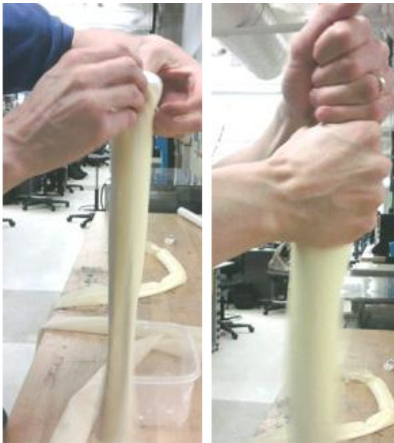
Figure 2. Use your hands to push and knead the silly putty mixture into the latex tubes.
