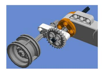
$\boldsymbol{B}$  Wheel is connected to larger gear on the left.
