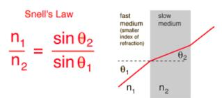
13. Find the indices of refraction of the liquids used and enter them into the data table. Remember, because air is the first medium, the index of incidence (n1) will be 1.00.
