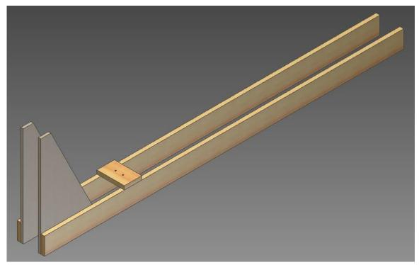
Use glue and 4-6 screws to attach the bucket base, flush with the rear of the 1x4, and center.
