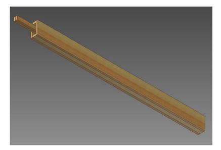
Attach the two 12" long 1x2s to the tower as shown, using glue and screws. Make sure that the two pieces are aligned and flush to the top of the 1x6s:
