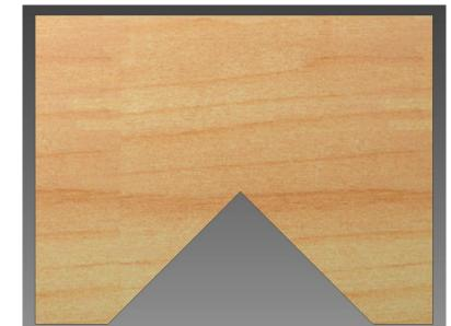
Attach the notched 1x4 pieces to the 34" 1x2s with glue and 2 screws per 1x2.
