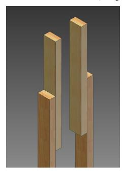
Spread a generous amount of glue on each surface and clamp them together, making absolutely sure that the edges of the boards are parallel. You may want to clamp them down to a flat piece of wood covered with wax paper or parchment paper to ensure that they are straight. Wipe off the excess glue that squeezes out (if none does, you didn't use enough glue) and leave the clamps on overnight.
