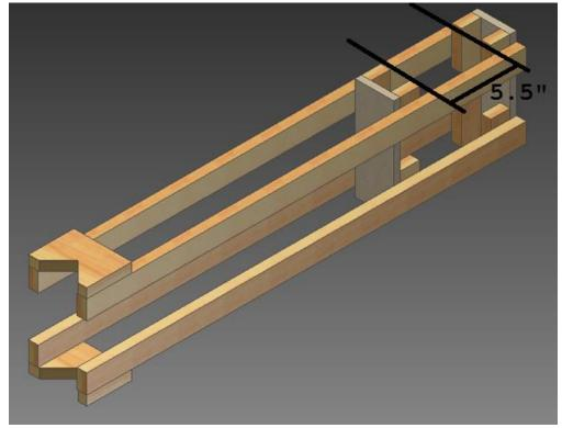
The easiest way to ensure the right spacing is to assemble the slider while the rub rail assemblies are clamped to the Lower Tower as shown:
