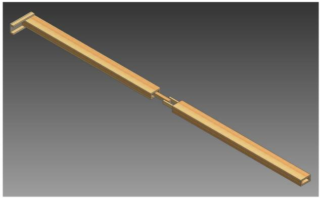
They might be very difficult to slide together. Make sure the two pieces are going in straight. If it is still difficult to slide them together, lightly sand the protruding 1x2s until you can push the two tower piece all the way against each other. Do not sand too aggressively; a tight fight is desired. Light mallet blows might be required, but it should not be so tight as to be impossible to disassemble.
