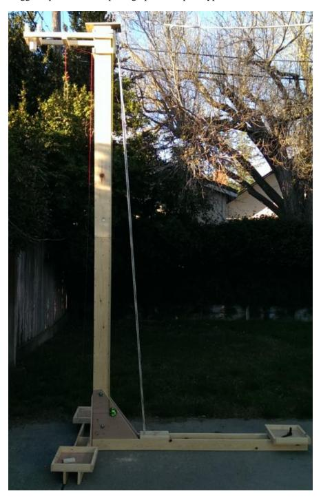
Without this egg dropper device, students must climb a ladder to drop the eggs. Using a ladder, the maximum drop height is about 8' and requires students to dangle themselves precariously to aim the eggs. This project was conceived to bring a cool machine element to the contest, improve safety and eliminate the aiming skill required if a ladder is used.
