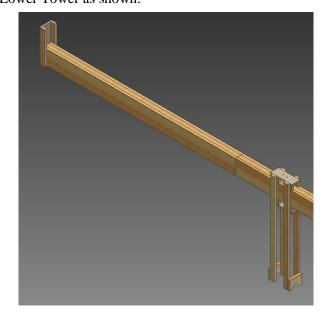
Move the slider up and down the Lower Tower. It should move freely but not loosely. If it will not fit on the end of the lower tower, sand the inside of the arms and rub rails that are interfering. Rounding over the upper and lower corners of the rub rails and arms helps the slider to move freely. This is probably the most critical part of the project and should be done very carefully. If you sand too much, you will need to remake the Slider.
