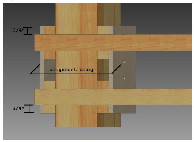
Wrap the Lower Tower with one layer of wax or parchment paper so you do not accidentally glue the slider to the tower. Align the rub rails and clamp them to the tower. Smear plenty of glue on the arms and rub rails then drive one screw into each rub rail/arm pair.
