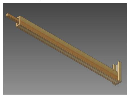
Drill two  $\frac{1}{4}$ " holes for installing the U-bolt with the 2 extra nuts and washers. Make the holes about 2" away from the edge of the board. The U side faces down toward the other side of the Upper Tower.
