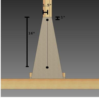
Use two 7" 3/8-16 bolts with nuts and washers to attach the Front Brace.
