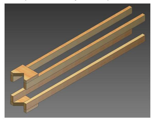
Glue the arms to the rub rails. The spacing between the rub rails is critical. Make the distance 5.5" as in the drawing:
