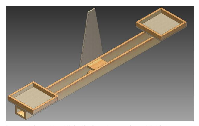
The screws might protrude into the inside of the beam. These tips can be cut off with a hacksaw or Dremel tool.
