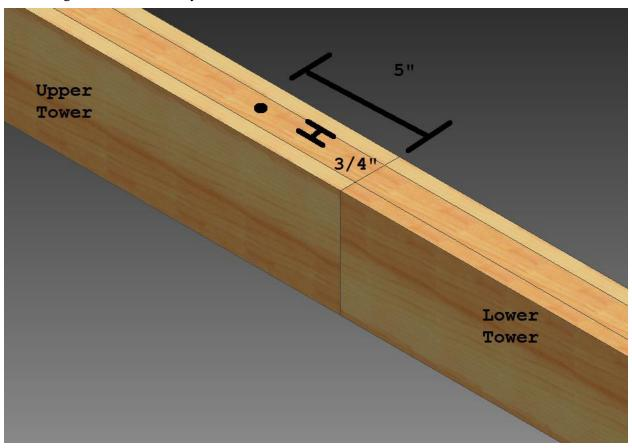
It is very important that this hole is drilled straight. Make sure that you will not be drilling through a wood screw.
