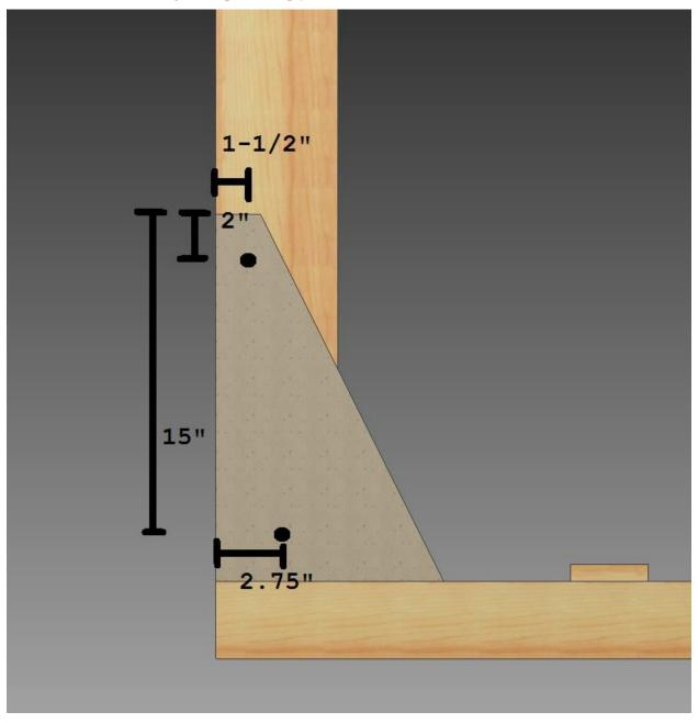
Use two 5" 3/8-16 bolts with nuts and washers to attach the rear brace to the lower tower.
