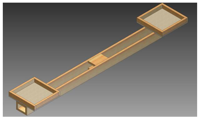
Mark the center of the beam, and the center of the bottom of the plywood trapezoid. Smear glue onto both parts, line up the center marks, and use 6-8 wood screws to attach them.
