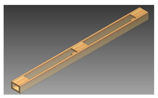
Add the bucket stands with glue and screws. The outside edges of the bucket stands line up with the ends of the 6' 1x6s. The bucket stands should be centered on the beam, but this is not critical.
