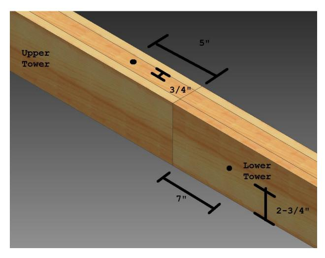
Add a 3-1/2" 3/8-16 bolt with a nut and two washers. Slide the Slider onto the Lower Tower as shown.
