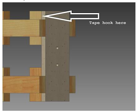
Let the tape measure hang down to the plywood triangle on the rear brace and mark this location. It will be somewhere near the tape measure in this picture:
