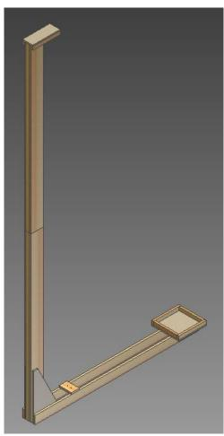
Use a corner level to ensure that the tower is plumb, and bump the rear brace until it sits flush with the front of the tower. Use two clamps to hold the tower to the Rear Brace and have your assistant hold the tower from falling over.
