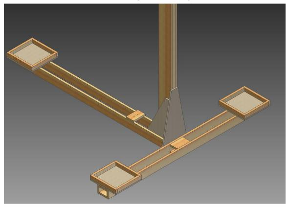
Drill two 3/8" holes through the plywood and all the way through the tower. Make sure you are not going to drill through a wood screw. The holes should be as shown:
