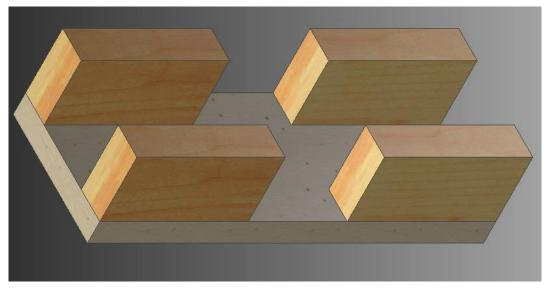
Cut a square corner out of the long side of the 4.5" 1x4s. Make the back of the corner about 2" from the flat edge.
