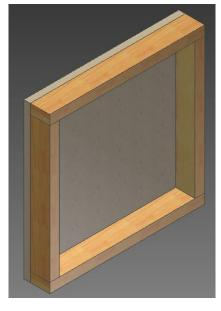
Assemble the beam using glue and 2 screws per 6" spacer as shown. Make sure the center of the two middle spacers is aligned with the center of the 6' 1x4.
