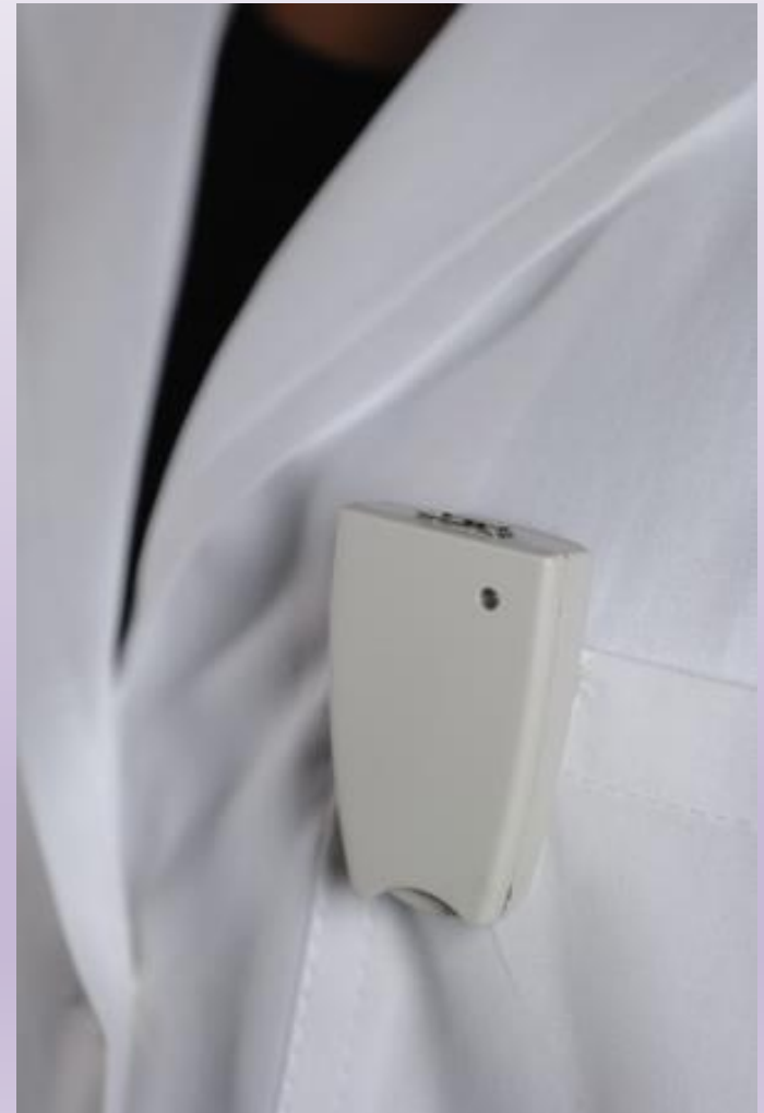
Pocket dosimeter; a NMR monitoring device with three Hall-effect sensors
