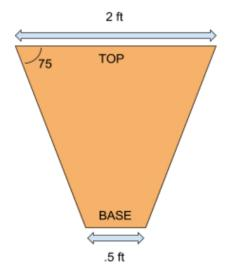
Answer: You need a total of 6 blocks in order to make the arch. The 2 blocks on the bottom of the arch will be half blocks in order to make sure the outside and inside of the arch at the ends are perpendicular to the ground.
