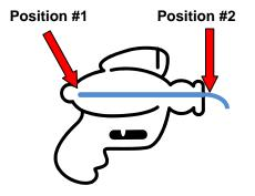
For the example problem given above, find the water pressure inside the gun  $(P_1)$ . [Hints: We know that the velocity of the water inside the gun  $(v_1)$  is initially zero, the pressure outside the gun  $(P_2)$  is the atmospheric pressure, or approximately 101,000 Pa, the density  $(\rho)$  is the density of water, and the relative heights  $(h_1 \text{ and } h_2)$  are equal because we are keeping the gun level.] Show your work in the space below:
