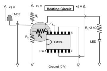
19. Now you can use Ohm's Law (V = RI) and your understanding of series circuits to develop an equation for  $R_4$ . Let's begin by looking at the voltage drop through  $R_2$  and  $R_4$  when the LED is lit.
