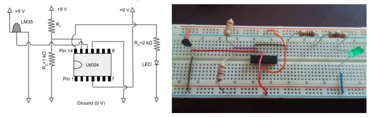
9. Connect the 9 V battery to the circuit and measure the voltage across R<sub>2</sub>. Is it still at your desired value? (Remember to disconnect the battery between measurements).
