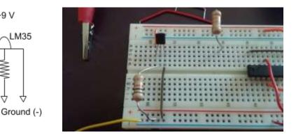
With a multimeter, measure the voltage across the 1 k $\Omega$  resistor. You should get a positive value 2. around 0.23 V. Rub your hands together and touch the top of the LM35 sensor. What happens to the voltage reading?
