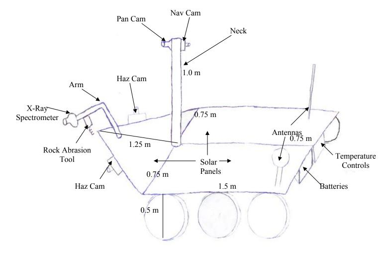
will sit on the wheels, where the required components will go, etc. Label the parts of your Rover and the dimensions of the major parts.
