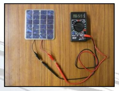
5. Turn the multimeter to measure current in the 20mA DCA setting. Note: Some multimeters use a squiggly line to symbolize AC (~) and a straight line to symbolize DC (—).
