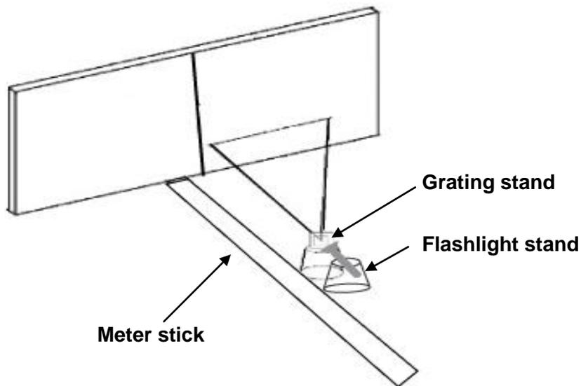
4. Place the flashlight stand directly behind the grating stand facing the screen. Rest the head of the flashlight on the grating stand so the beam of light travels directly through the center of the grating.
