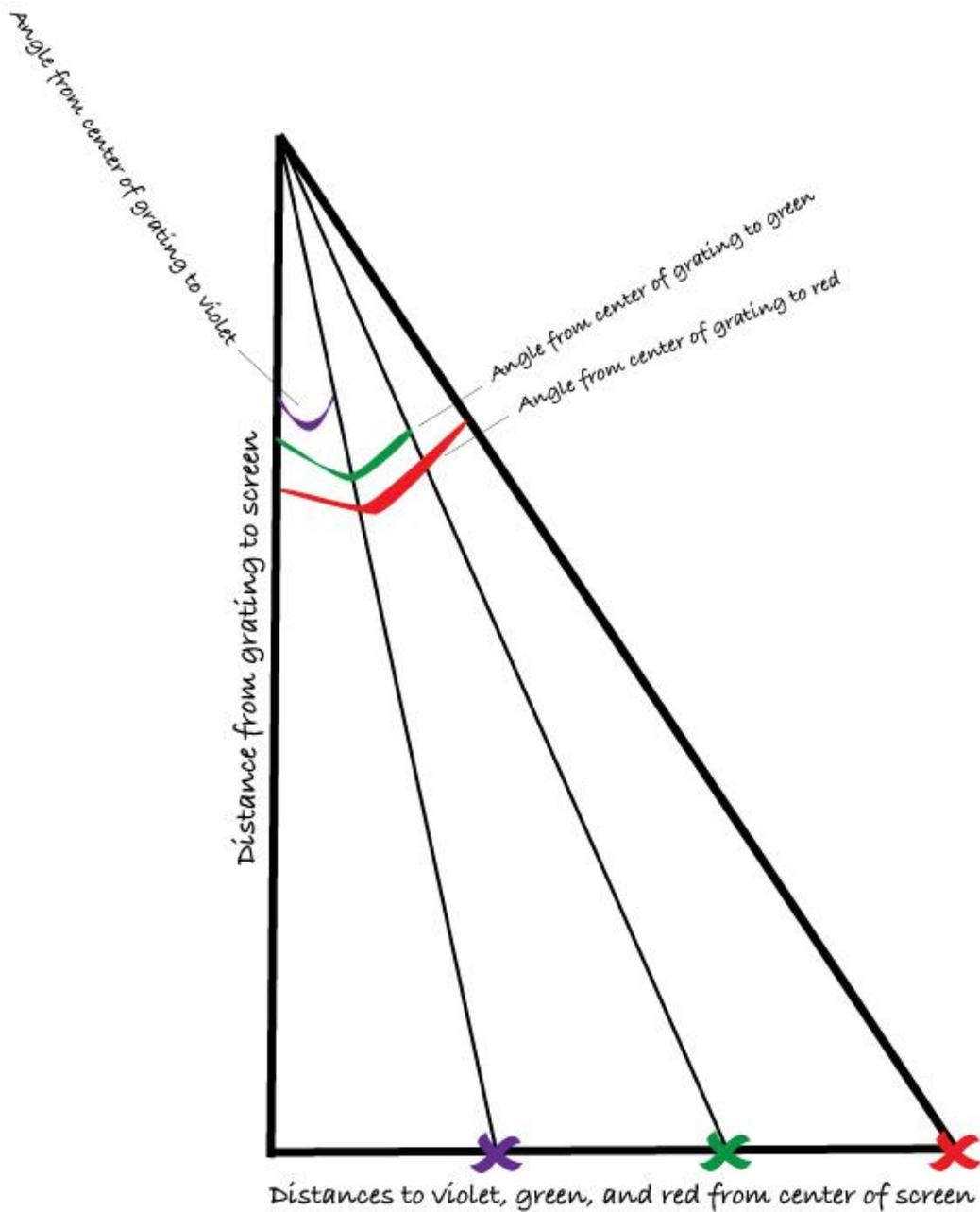
11. Using a protractor, measure and record the angles to each color.
