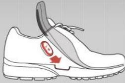
Place the sensor in your left Nike+ shoe, in the built-in pocket beneath the insole. You can leave the sensor in your shoe even when you're not working out.
