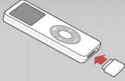
Attach the receiver to your iPod nano. The receiver fits snugly into the Dock connector, located on the bottom of your iPod nano next to the headphone jack.
