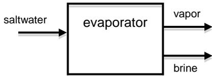
**Evaporator:** This component takes in saltwater and produces water vapor and brine.
