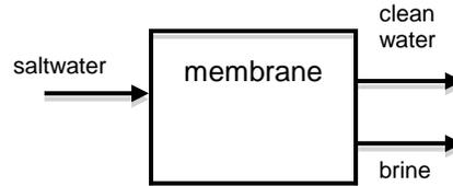
**Membrane:** This component takes in saltwater and pushes it through a membrane capable of removing salt ions. It produces clean water and brine.
