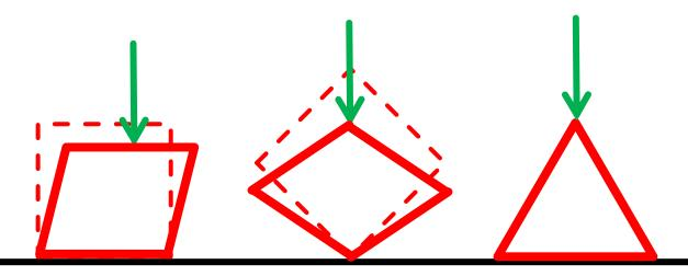
The other shapes collapse because the angles between the structural members change.
