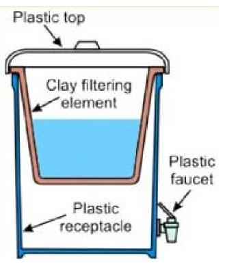
particles. Candle filters are wiped clean and boiled and then checked for cracks and fissures. Filters coated in colloidal silver need to be recoated approximately once per year.
