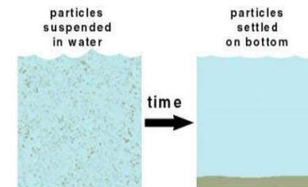
**Figure 3.** [Sedimentation Process](#).
