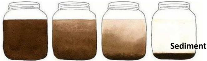
**Figure 1.** Sedimentation of muddy water.
