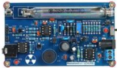
Assembled Radiation Detector System
