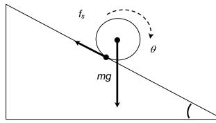
A spherical rigid body of mass *m* is rolling down an incline surface. The forces producing this movement are the weight of the body mg and the force of friction  $f_s$ .
