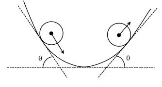
A sphere rolling on a path with variable slope can be visualized as rolling on a sequence of inclined tangent straight surfaces.
