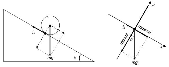
The forces that make this spherical solid of radius *r* and mass *m* roll down the incline plane are those along the *x*-axis. Using Newton's second law to describe the solids linear movement:
