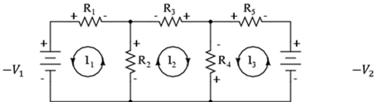
**Part 1:** Using a TiNspire calculator, solve the following three equations with three unknown variables. The three unknowns are the currents represented by  $I_1$ ,  $I_2$ , and  $I_3$ , as illustrated above.
