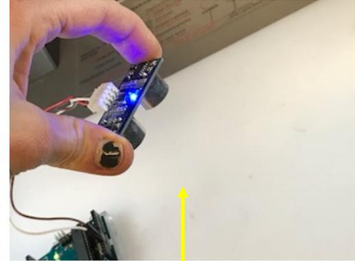
The receiver should point in the direction of the object
