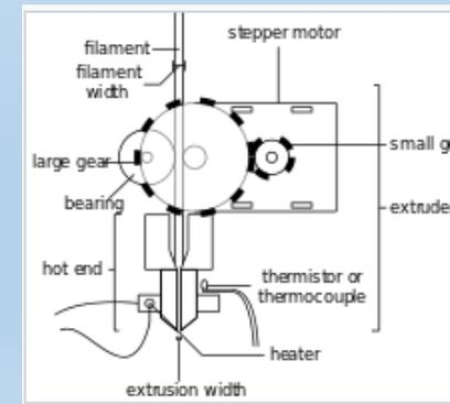
Image 1: Cutaway of extruder and motor
