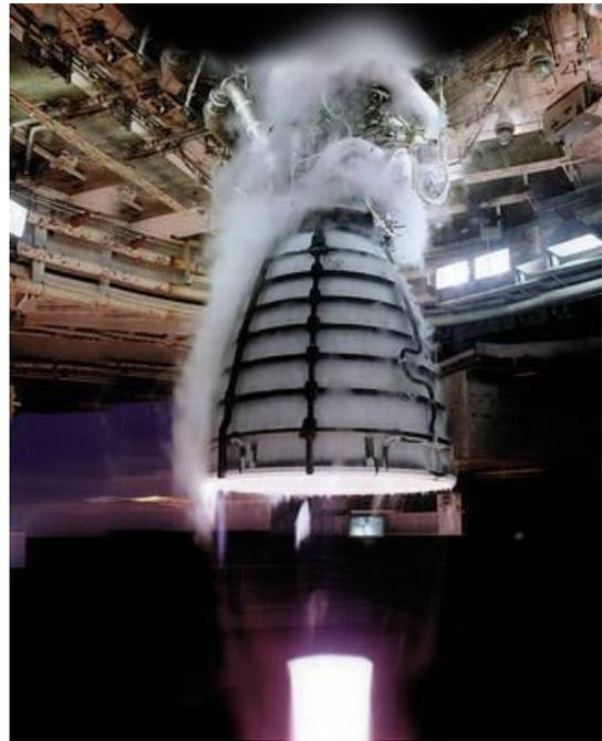
Four RS-25 engines, like the one pictured above undergoing a hot-fire test, power the core stage of NASA’s Space Launch System (SLS)—NASA’s heavy-lift launch vehicle.
