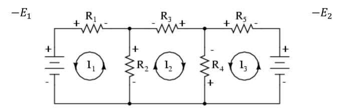
Either by hand or using a Ti-Nspire calculator, solve the following three equations with three unknown variables. The three unknowns are the currents represented by  $I_1$ ,  $I_2$ , and  $I_3$ , as illustrated above.
