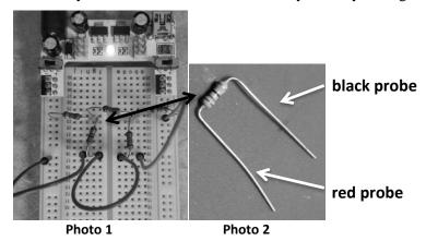
*Photo 1* shows an experimental circuit that is the real electrical circuit for the previous schematic diagram. The resistors are lined up in the same way. If you are not sure, please ask for help.
