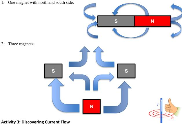
Draw a picture that illustrates your finding for the current flow. When turning the crank clockwise, current flows from the positive + (red) wire to the negative + (black) wire. Use the right-hand rule to show the resulting magnetic field flow for each direction of current flow. Point your compass toward north.
