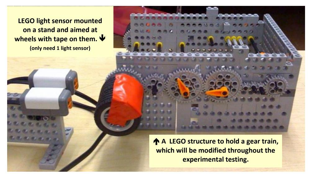
Gears: Determining Angular Velocity Activity—Example Experimental Setup Visual Aid
