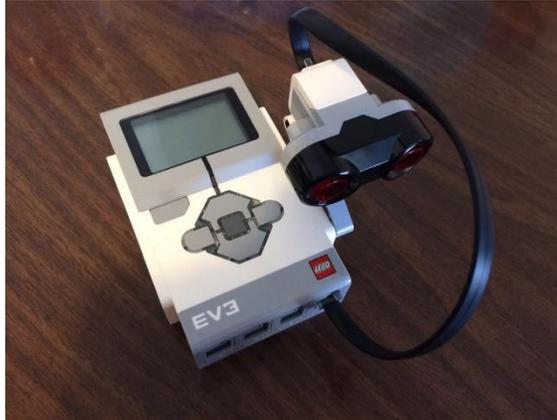
Figure 1: Alternate EV3 sensor setup, with brick and attached ultrasonic sensor.
