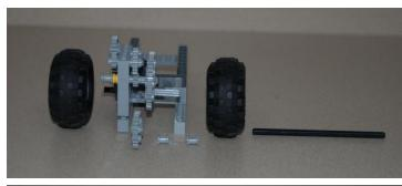
17. Add wheels to the gear box using the pieces shown at left.
