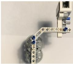
18. Mount the angle indicator using the connector and axle. Be sure to fit the color sensor through the holes.
