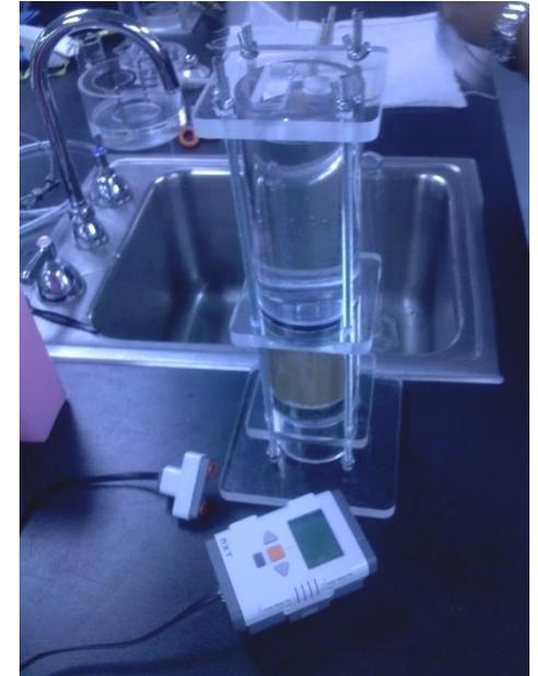
Permeameter with ultrasonic sensor and EV3 to measure water volume and time
