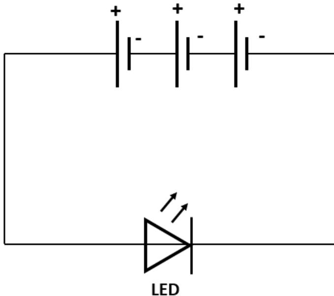
7. Draw a diagram of the circuit that produced the correct amount of voltage and current to turn on the LED light bulb.
