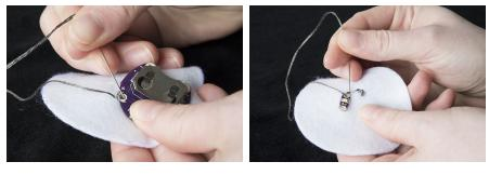
using a straight stitch, follow your path to the next positive hole on your LED. Don't forget to loop 3-4 times on each hole to secure. Once you have finished at the LED, tie a knot in your thread and trim any excess. Congratulations, you've just sewn the first part half of your circuit!
