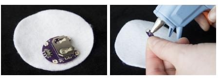
not on top of the battery holder. Make sure the + and - symbols line up with the symbols on the battery holder. Be careful not to cover the holes with glue – we'll need those to sew through later. *Do not put your battery in yet.*
