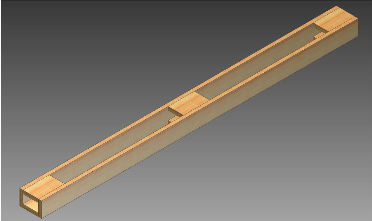
Add the bucket stands with glue and screws. The outside edges of the bucket stands line up with the ends of the 6' 1x6s. The bucket stands should be centered on the beam, but this is not critical.
