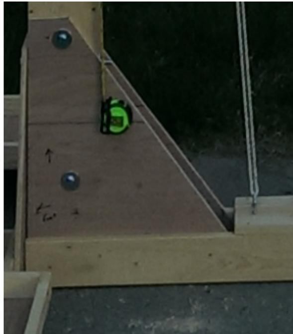
Drill 4 holes at the corners of the tape measure, and secure it in place with zip ties.
