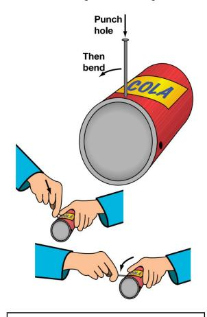
**Tip** Make sure the nails used for punching holes have good points on them. They do not have to be needle sharp, just not blunt.
