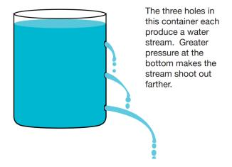
The effects of the other variables are many. For example, more holes means more water streams out of the can, but the water drains from the can more quickly. Large holes drain water more quickly than small holes. Holes angled in different directions counteract each other. Holes that are not angled produce water streams that leave the can perpendicular and no rotation occurs. (The object is to have students discover the effects of the different variables themselves.)
