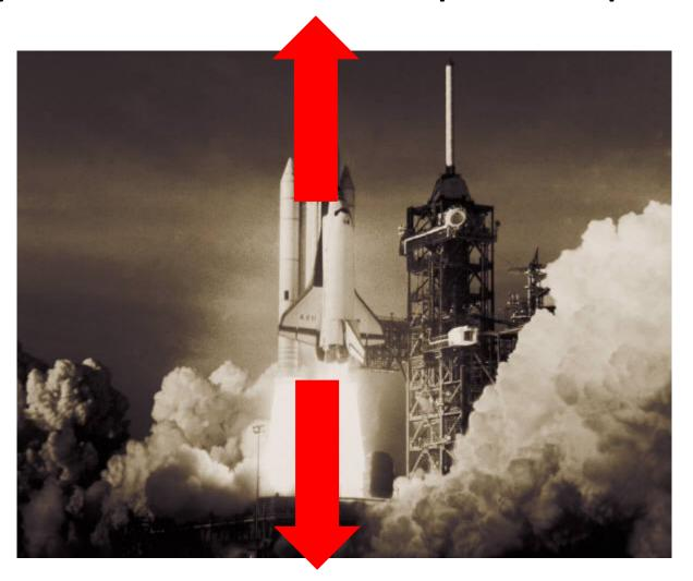
The space shuttle exerts a force downward, and the reaction force pushes it upward.
