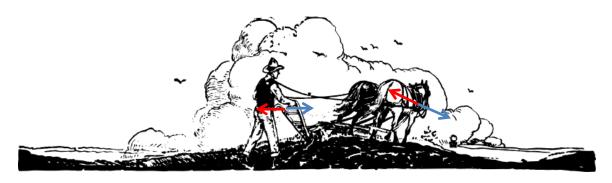
The horses pull the ropes (to the right) (blue arrow), and the ropes pull back on the horses (to the left) (red arrow). Similarly, the ropes pull the man and his plow forward (to the right) (blue arrow), and the man and the plow pull backwards against this to (to the left) (red arrow). Note that another force pair could be drawn in the soil, between the plow and the soil.
