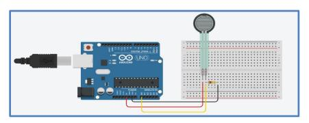
breadboard. Connect the other end of the 10 k $\Omega$  resistor to the microcontroller's analog input (A0).
