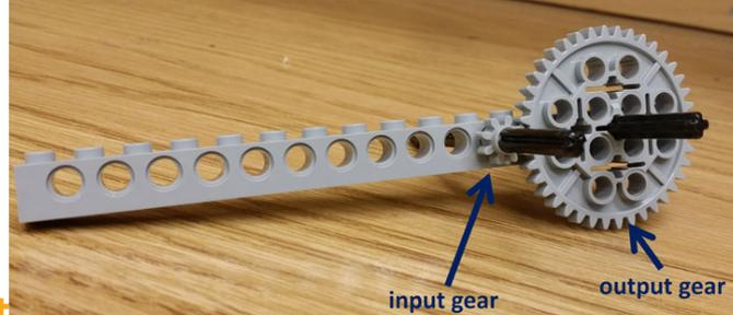
In this case, the gear ratio is defined as  $1:X$  (output:input). Notice that this is in the same ratio as the number of teeth, that is, 8:40 or 1:5.
